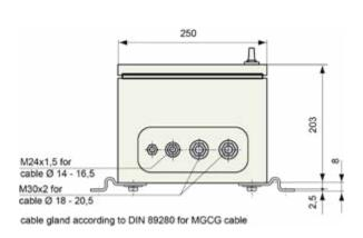
Standard control box (supply voltage 380 / 440 V - control voltage 115 / 220 V) - other voltages on request weight approx. 8,7 kg  $\,$
